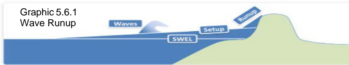
The storm surge stillwater elevation (SWEL) and added effects of wave setup
